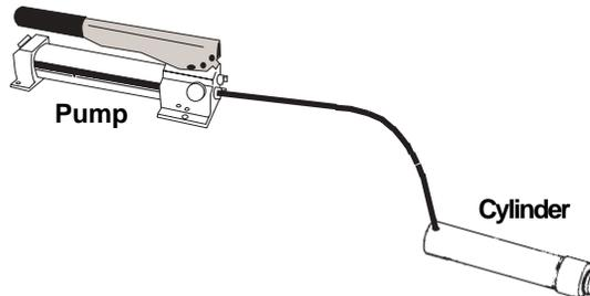
**IMPORTANT: Some spring return cylinders, or rams, have a cavity in the rod which forms an air pocket. This type of cylinder or ram should be bled when positioned upside down or lying on its side with the port facing upward.**
